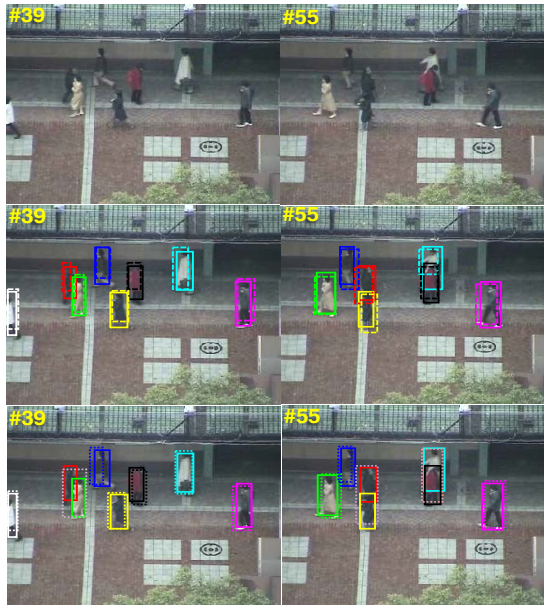
Fig. 10. Examples of tracking results under partial occlusion. The 1st row is the original frame images, the 2nd and 3rd rows are the results comparing our algorithm with ZG and YG algorithms respectively.
